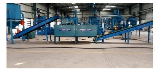
5. Eldan line Input Conveyor with Rasper
